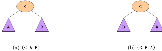
Fig. 8 Two less-than expressions, with identical children in reverse order. (a) is not equivalent to the negation of (b) since both return false in the case of A and B returning the same value.
