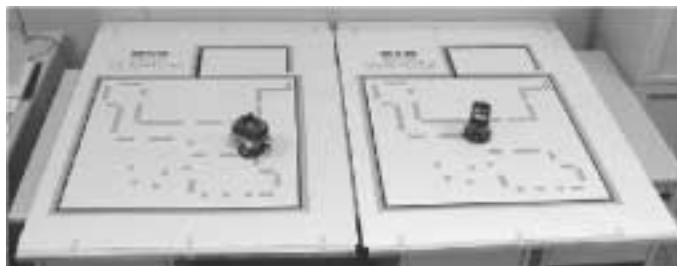
Figure 1: The Lausanne trail experimental setup. We added a special track enclosing the environment, which is used to guide the robot back to the starting point.
