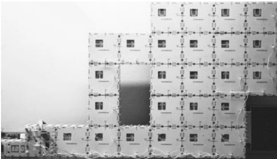
Figure 9: Beuchat and Haenni: hardware implementation of one of the organs of von Neumann's universal constructor, known as a pulser, using the module of Figure 8. The above pulser P(11001) generates at the output cell (top right) the sequence of excitations (signals) 11001 a fixed number of time steps after receiving an excitation (i.e., a 1 signal) at the input cell (bottom left). Note that the 25 von Neumann modules are not arranged as a 5 \times 5 square – in fact, the arrangement is that of a 7 \times 7 square, where unused cells are simply not implemented. This allows for the construction of a larger organ for the price (literally) of a smaller one.
